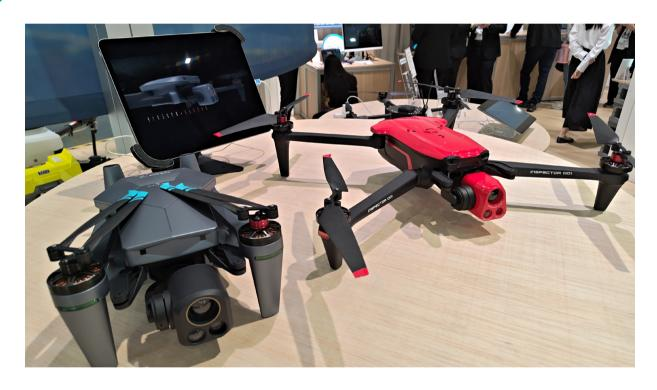
During COMPUTEX 2025, the Qisda Smart UAV Business Unit introduced how their Scouting Drone utilized DFI's QRB812 for edge Al integration. The Scouting Drone uses infrared and dual cameras to enable heat and daylight vision. With the edge Al enabled by the QRB812, the Scouting Drone is able to do image recognition and object tracking.
